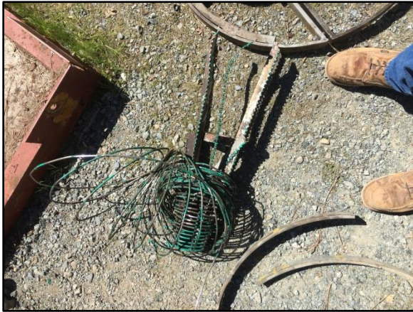
Damaged turbine pump filter screen
