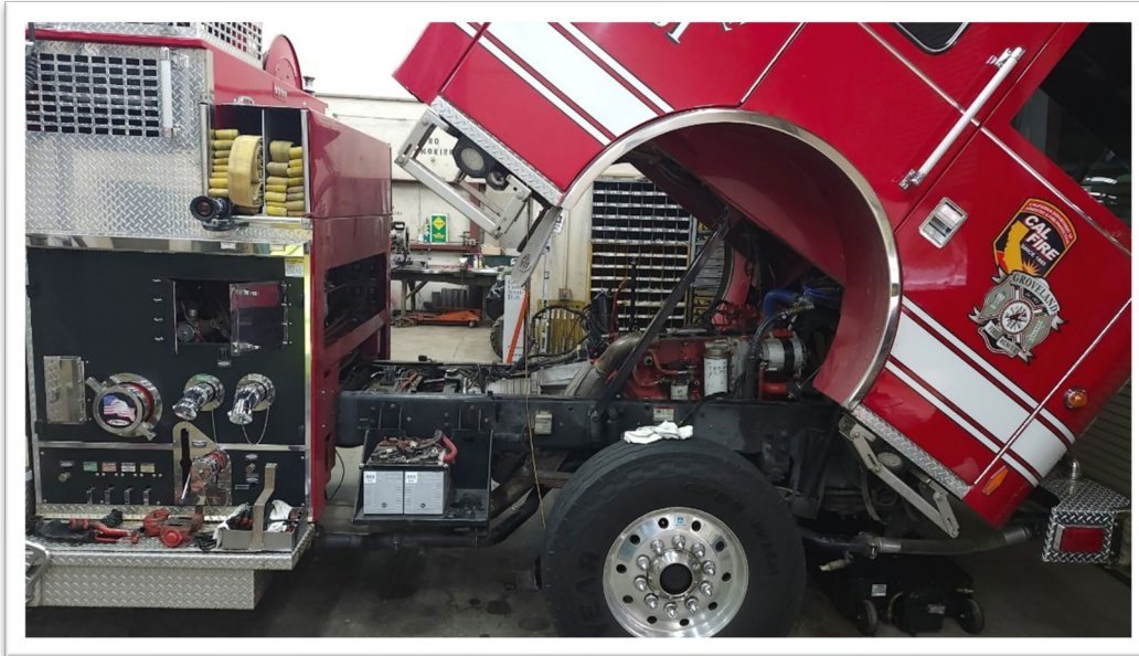
Engine 781 In-frame rebuild.
